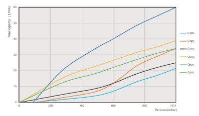
Note: Above data is based on the 220V/50Hz instrument
